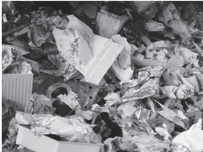
Chunk particle sizing - output from a PRI-MAX®
